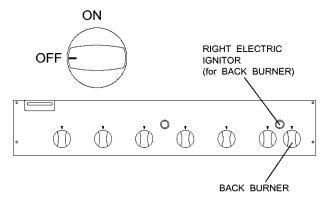
Immediately press the Right Electric Ignitor for 3-4 seconds to light the Back Burner.
